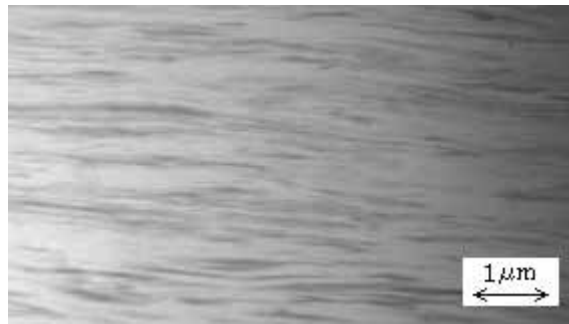
Figure 6. Transmission Electron Micrograph of Molding (TEM photo) Composed of PELECTRON PVH (10 wt %) and LDPE
