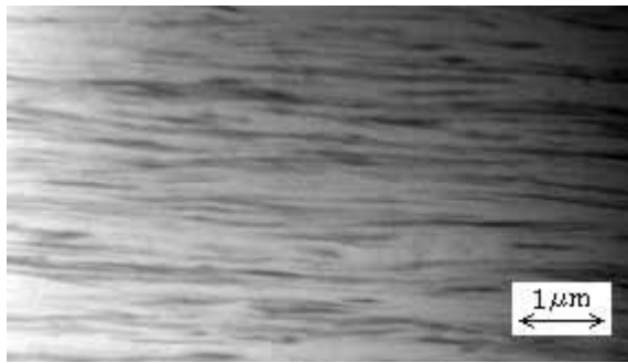
Figure 6. Transmission Electron Micrograph of Molding (TEM photo) Composed of PELESTAT 230 (10 wt %) and LDPE
